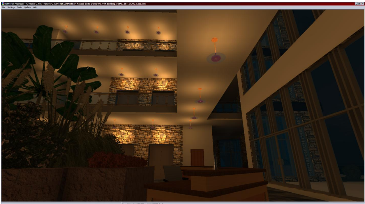
Light Map Type Ambient with all lighting fixtures included and Sun Settings Time set to 11:00pm (Lights are checked on in Light List and Bake local lights checked)
